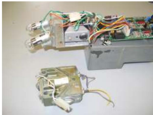
AMF scoring systems require voltage output to signal the scoring system and Brunswick requires a switch closure to signal the scoring system.
